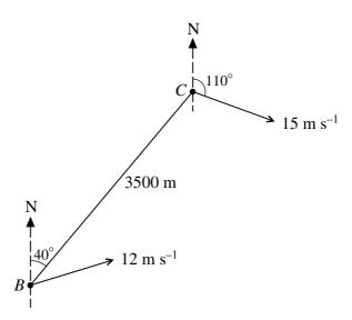
From a boat B, a cruiser C is observed 3500 m away on a bearing of 040°. The cruiser C is travelling with constant speed  $15 \,\mathrm{m\,s^{-1}}$  along a straight line course with bearing  $110^\circ$  (see diagram). The boat B travels with constant speed  $12 \,\mathrm{m\,s^{-1}}$  on a straight line course which takes it as close as possible to the cruiser C.
