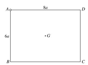
The diagram shows a uniform rectangular lamina ABCD with AB = 6a, AD = 8a and centre G. The mass of the lamina is m. The lamina rotates freely in a vertical plane about a fixed horizontal axis passing through A and perpendicular to the lamina.
